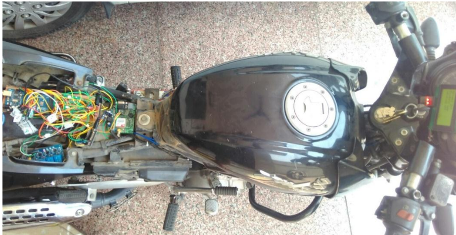
Figure 6- The hidden internal circuit installed in the bike
