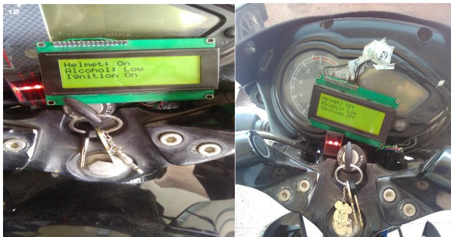
(a) LCD showing helmet ON (b) LCD showing helmet OFF
