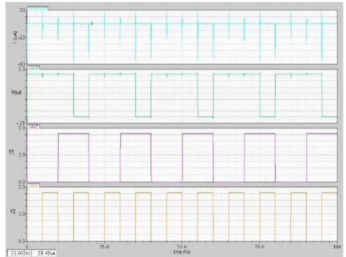
Fig 2. Transient Response of conventional NAND gate
