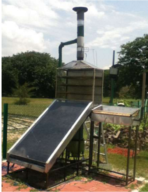
Fig. 15 Hybrid dryer test rig [127]
