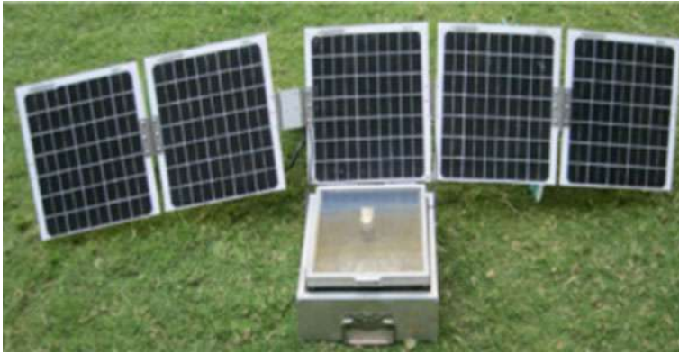
Fig. 11 Experimental setup of a hybrid solar cooker [103]
