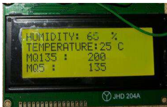
Fig.3: Data displayed on LCD display
