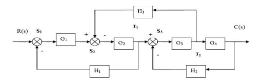
(b) Find overall transfer function using signal flow graph:
