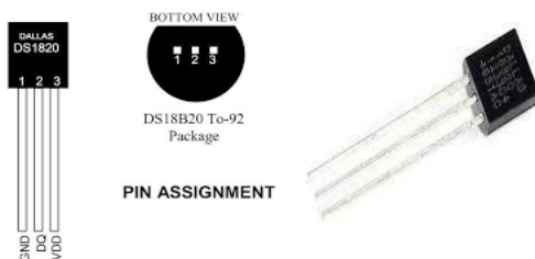
Fig 2: Temperature Sensor DS18B20
