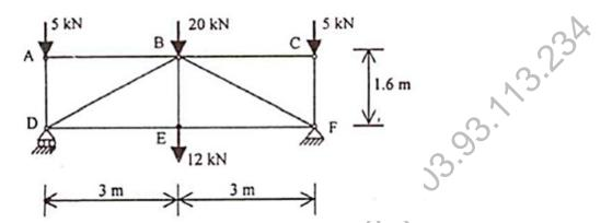
(b) Using method of section, determine the forces in the members of the trusses shown.
